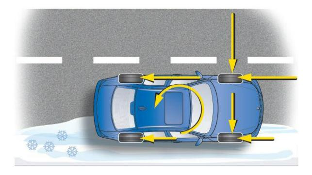
In the case of braking on different surface friction coefficients (asphalt/ice or snow), a moment builds up about the z or vertical axis (yaw moment) rendering the vehicle unstable. In this special case, the Active Steering control unit calculates the steering angle (maximum  $\pm 4^{\circ}$ ) required for the front wheels to keep the vehicle stable using the actual yaw rate and the longitudinal and lateral acceleration.
